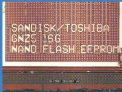
Toshiba 56nm 16Gb MLC NAND Flash Part Die Markings
