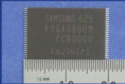
Counterfeit Samsung Part Package Marking K9GA08U0M
