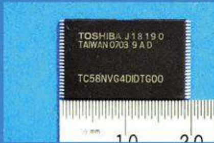
Counterfeit Toshiba Part Package Marking TC58NVG4D1DTG00
